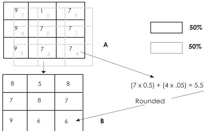
Figure 3: Weighted overlay procedure
