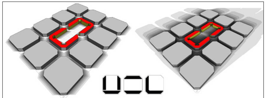
Figure 4: A sun and shading extent study of the originally planned Barcelona 4 storey manzanas illustrated in Figure 3. The image on the left is for 20 June (summer solstice) and on the right 21 December (winter solstice). The diagram in the middle illustrates some of the block configurations that Cerda originally had in mind.
