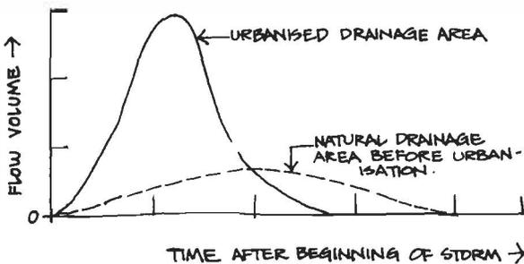
SCHEMATIC HYDROGRAPH SHOWING RUNOFF CHARACTERISTICS BEFORE, AND AFTER URBANISATION WITHOUT STORMWATER ATTENUATION:
