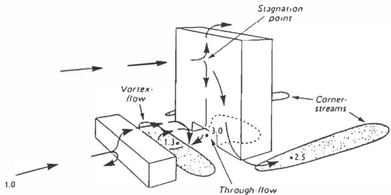
FIGURE 1.2. *Air flow around a tall building with lower buildings upwind. The three main regions of increased wind speed at pedestrian level (stippled) are illustrated, see the text for the meaning of the numbers. Source: Oke, 1978.*
