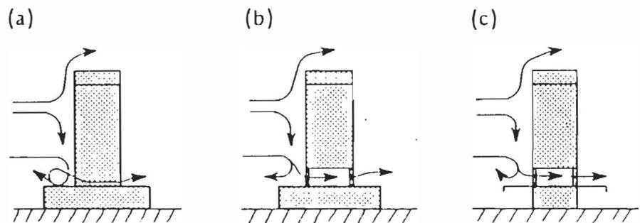
FIGURE 7. Tall building designs helpful in alleviating undesirably increased wind speeds at pedestrian level (modified after Hanlon, 1972).
