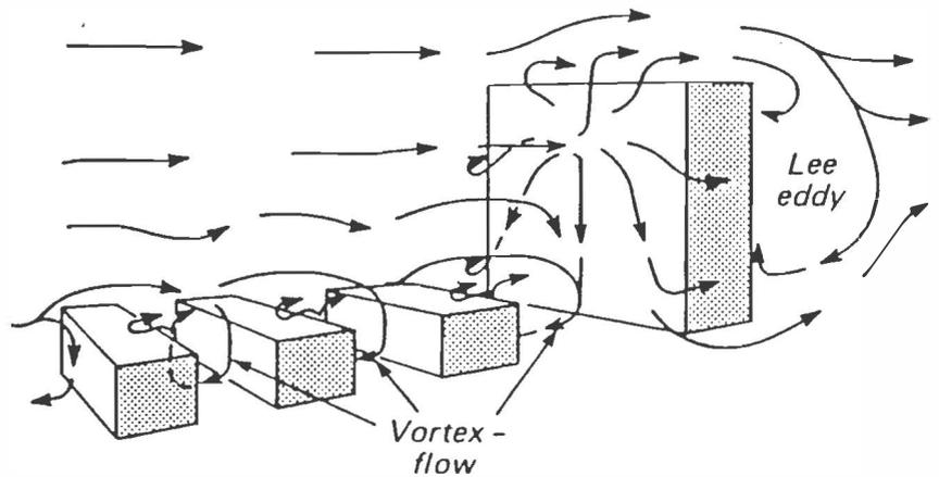
FIGURE 1.1. *Flow patterns over and between buildings of approximately the same height (left) and in the vicinity of a relatively much taller building (right). Source: Oke, 1978.*
