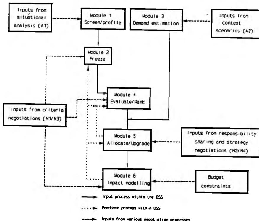
FIGURE 3: *Modules of decision support system applied within a scenario-based approach.*
