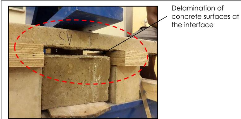
Figure 5: Precast and cast-in-situ concrete delaminates
