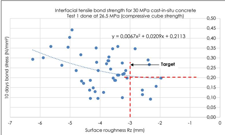
Figure 6: Interfacial tensile bond strength at ten days for 30 MPa concrete
