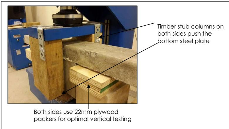
Figure 4: Specimen testing
