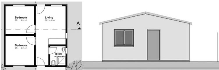
Figure 3: Plan and elevation of a typical 40m<sup>2</sup> RDP house
