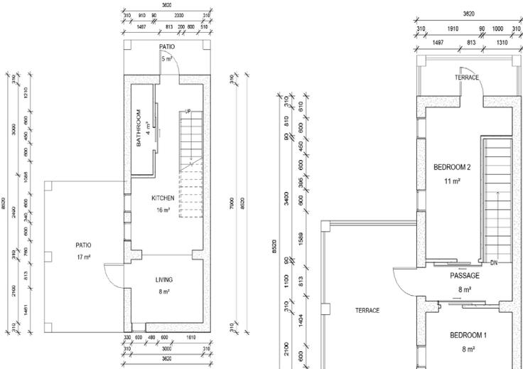
Figure 5: A 10X10 Sandbag House floor plans
