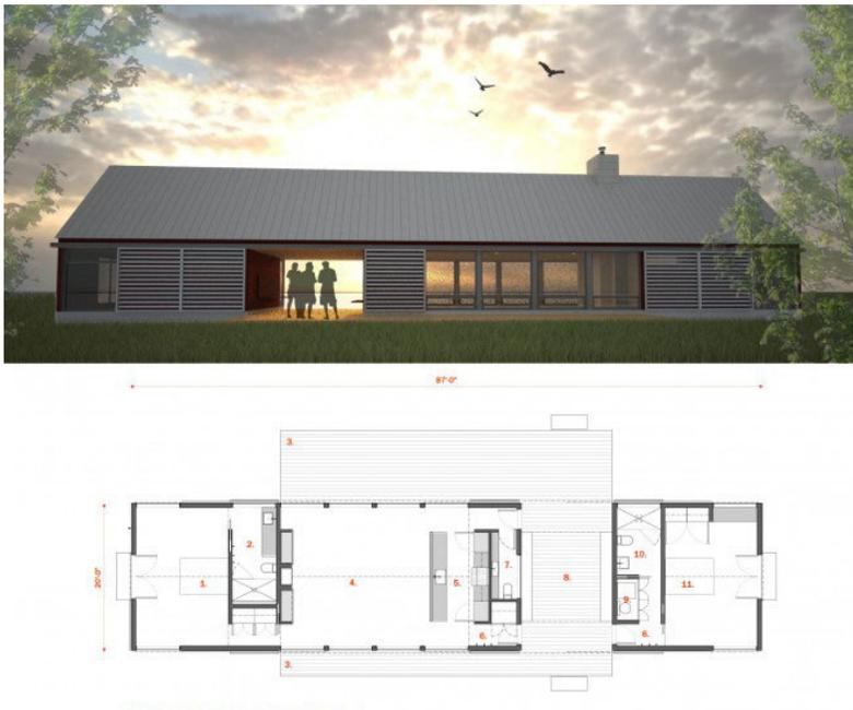
Figure 12: Productised Longhouse plan and elevation by Eric Reinholdt
