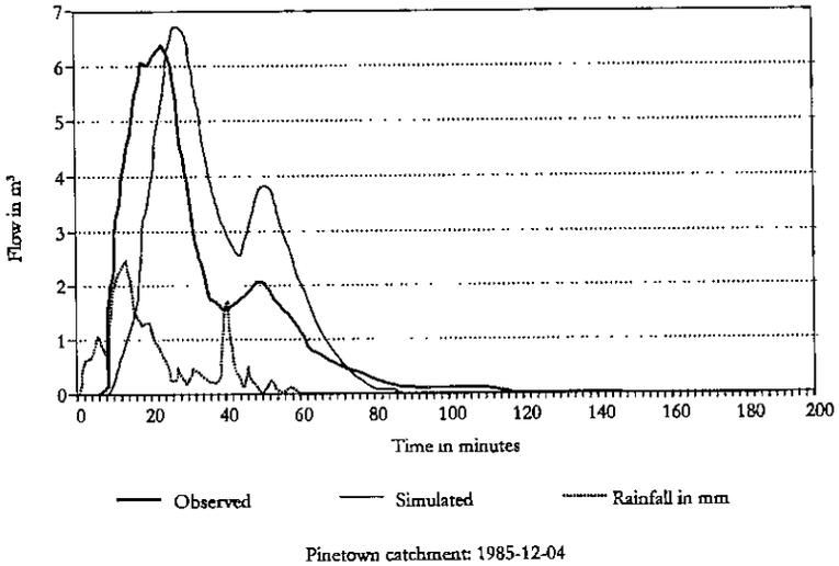
Figure 10: Simulated vs observed flow in the Pinetown catchment
