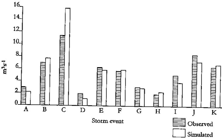
Figure 11: Simulated vs observed peak flow for selected storm events at Pinetown
