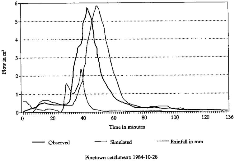
Figure 9: Simulated vs observed flow in the Pinetown catchment
